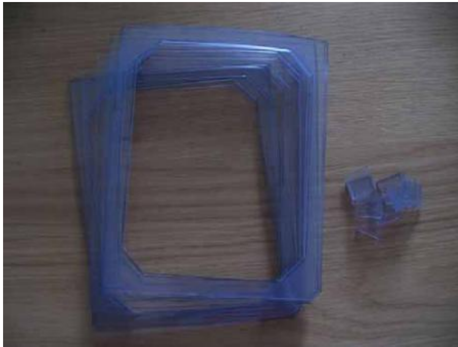
Figure 3. Soft PVC spacers rings
