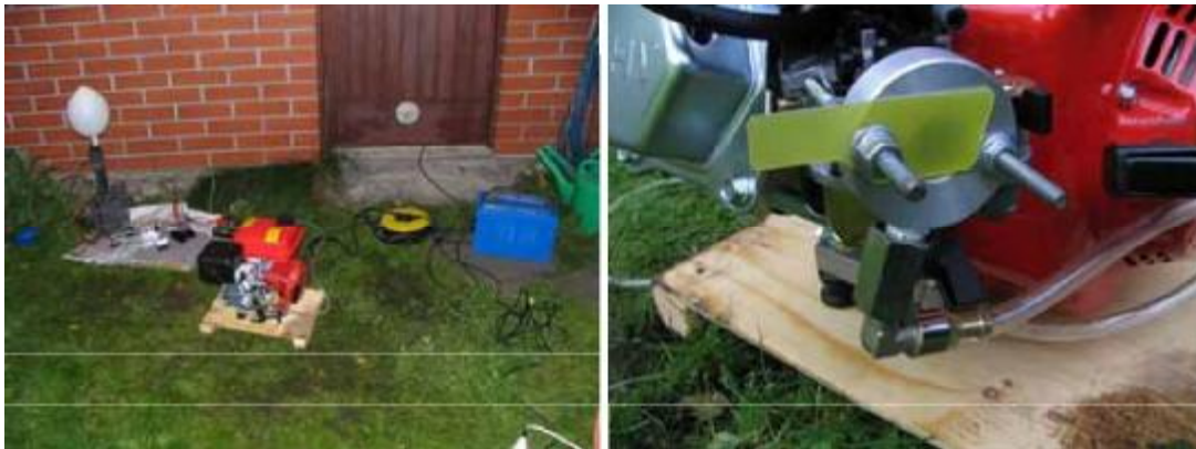
Figure 14. 6.5hp 200cc 4-stroke running on electrolytic gas
