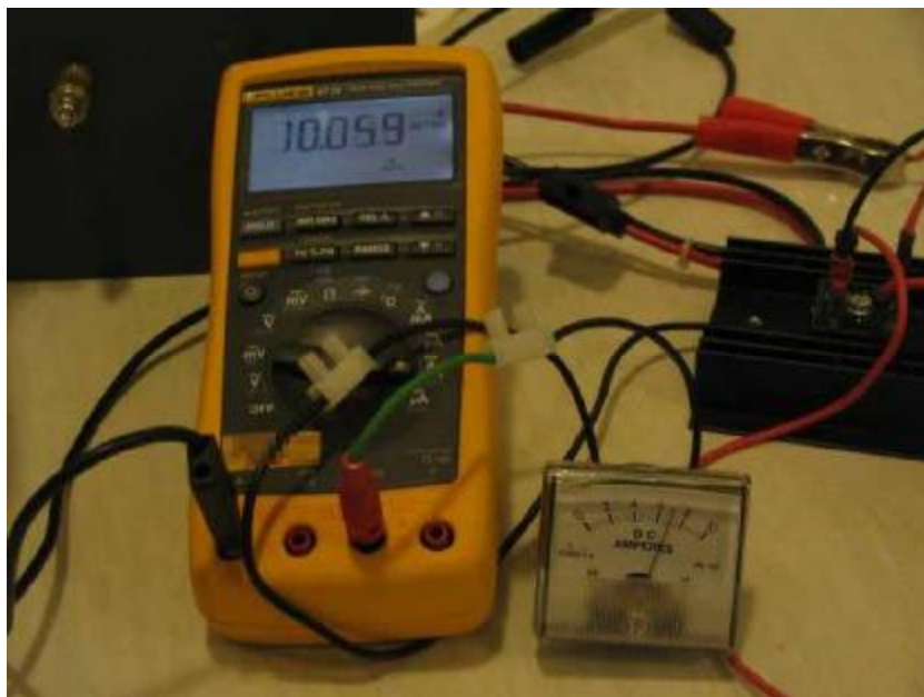
Figure 12. Comparison between current meter readings for pulsed electrolyzer current
