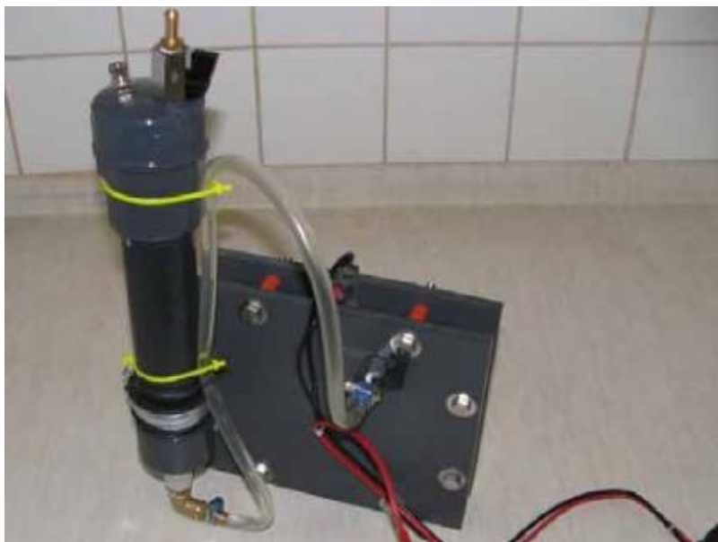
Figure 8. Finished electrolyzer with bubbler
