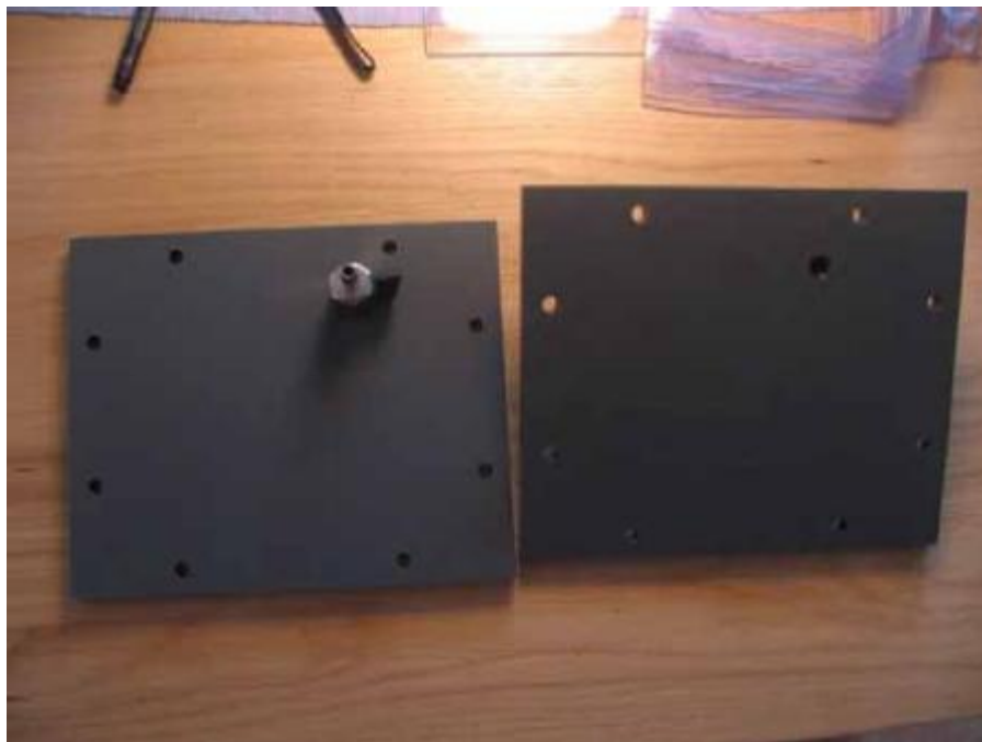
Figure 4. PVC end plates with gas valves attached
